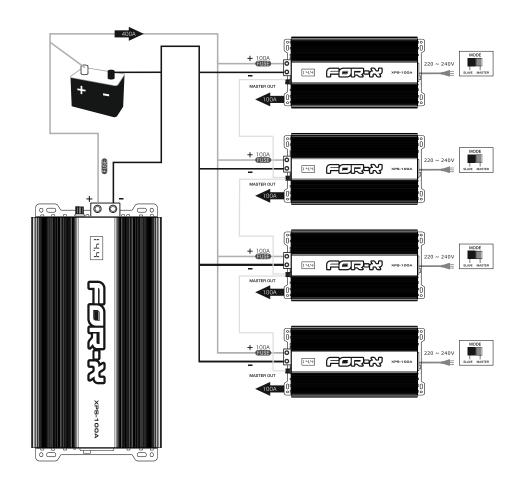
WARNING: Do not overload AC power outlets to avoid danger of electric shock and fire. A minimum current of 20A per XPS-100A will be required. Avoid connecting multiple power supplies to a single AC outlet using power strips.
