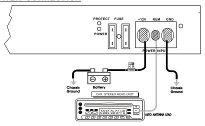
**IMPORTANT!** Before making any connections, disconnect the car's battery until the installation is completed to avoid possible damage to the electrical system
